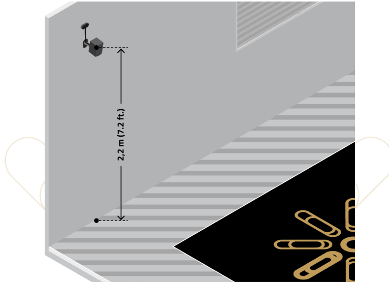
Figure 4 - Base station distance above the ground
